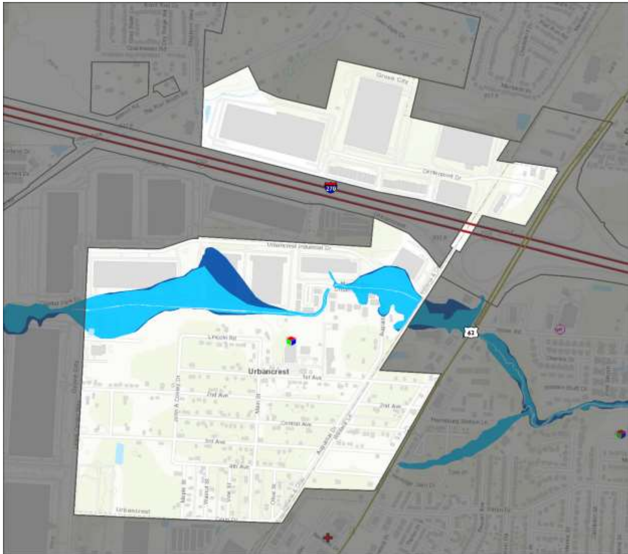
Figure 9.36-1. Village of Urbancrest Hazard Area Extent and Location Map – Flood
